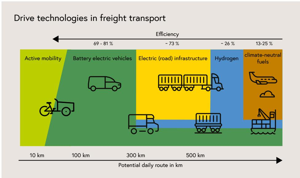
Figure 6 The role of the different drive technologies and their efficiency in freight transport
