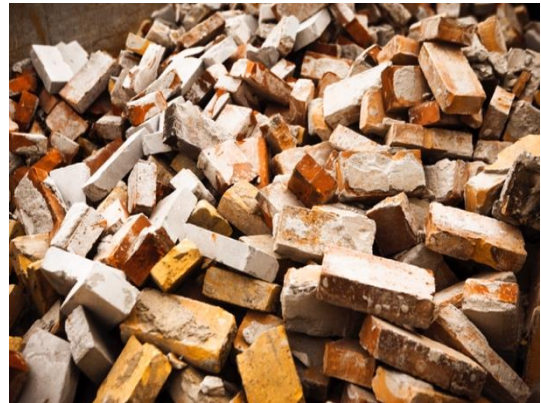
Figure 10 Preparing for re-use includes cleaning of bricks (Source: Danish Technological Institute)
